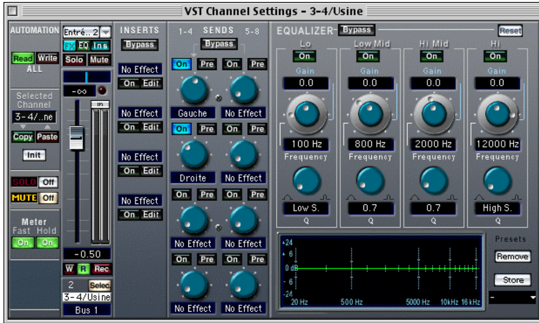
Fig 3 This configuration is without danger, since the "Pre" buttons on the effects are deactivated. We are thus in "post-fader" mode: by muting the track, the effect send will also be blocked.
