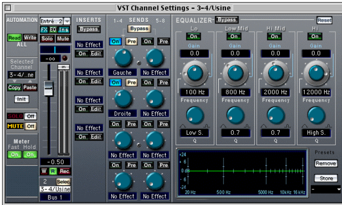
Fig 4 Here, to overcome the danger that the "Pre" output is being used, we have used the "Bypass" function, which will turn off all the effect sends from this track. This is confirmed by the fact that the "FX" indicator is dimmed.
